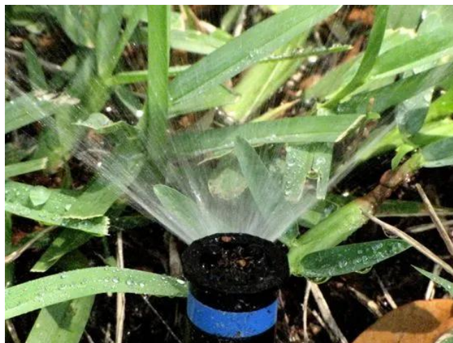
Figure 3. Standard head with a fixed spray nozzle. Credit: Bernard Cardenas, UF/IFAS
