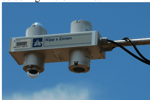
Figure 9. CNR-1 net radiometer
