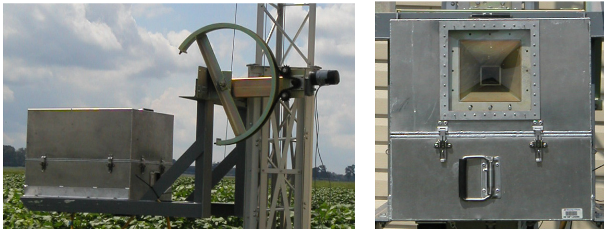
Figure 4 (b) and (c). The side view of the UFCMR showing the rotary system and the front view of the UFCMR showing the receiver antenna.
