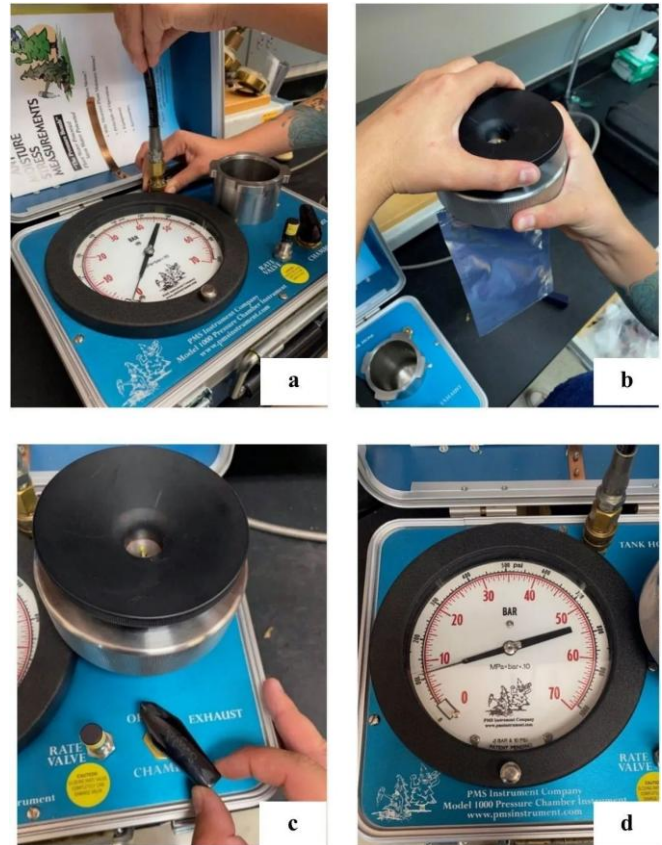
Figure 5. Steps (a–d) for measuring leaf water potential using the pressure “bomb” method. Credit: Christian Bartell, UF/IFAS
