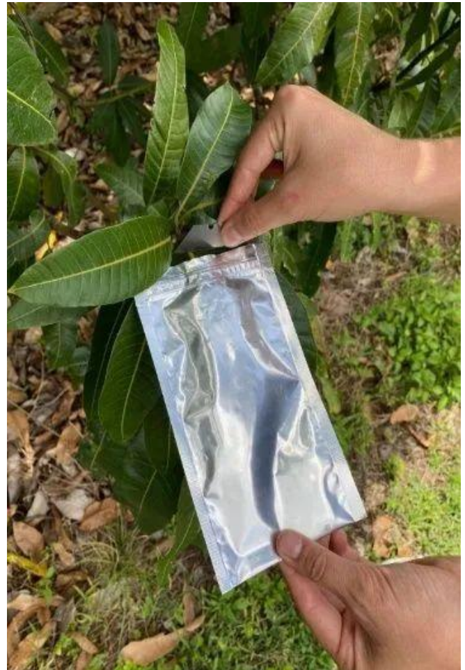
Figure 3. Covering a leaf sample with a reflective bag and cutting a leaf sample for measurement. Credit: Christian Bartell, UF/IFAS
