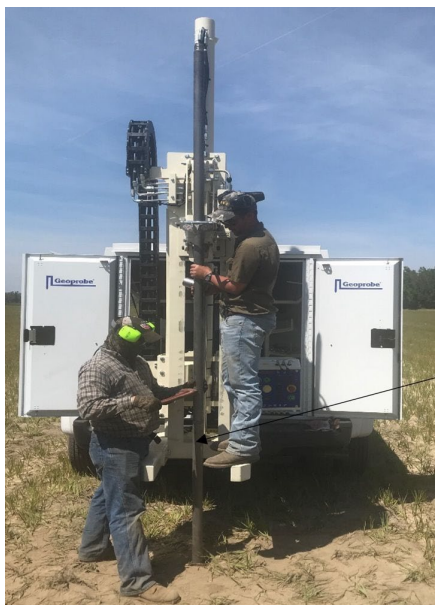
Figure 3. Geoprobe soil sampling carried out in Malone, FL.
