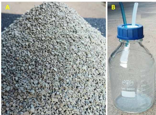
Figure 5. A) Grouting bentonite used as a sealant. B) Sampling bottle used to collect soil solution. Credit: Bibek Acharya and Dr. Vivek Sharma, UF/IFAS
