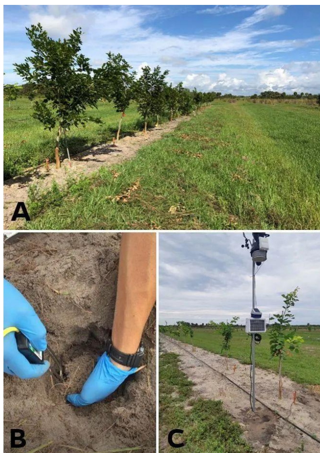
Figure 2. Field trial located at the UF/IFAS Indian River Research and Education Center (UF/IFAS IRREC) in Fort Pierce, FL. (A) Two-year-old pongamia trees at the UF/IFAS IRREC field trial. (B) Installation of a soil moisture sensor in proximity to pongamia roots. (C) Weather station that measures evapotranspiration and transfers the data to a computer server.
