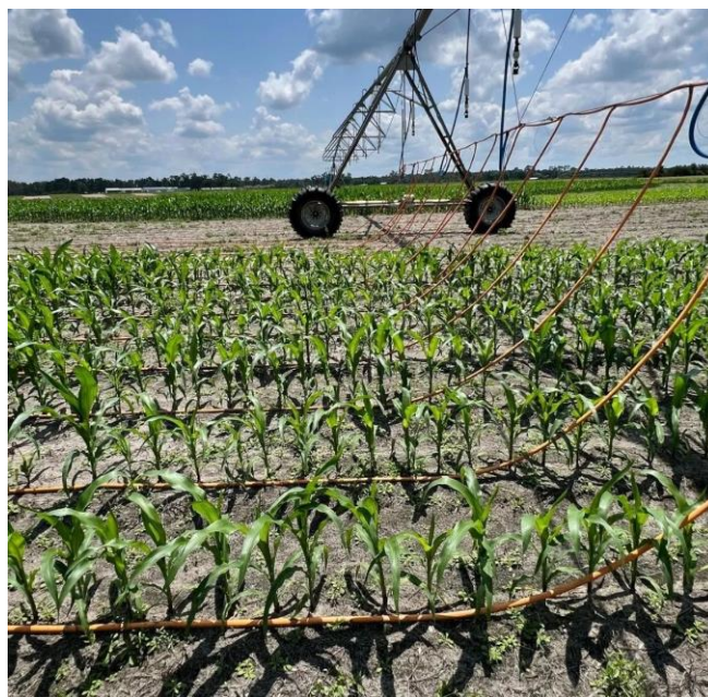
Figure 1. A center pivot irrigation system equipped with mobile drip irrigation technology at Live Oak, FL.
