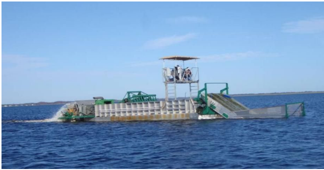
Figure 8. Mechanical harvester with hydraulically driven paddle wheels in the back and articulated cutter/conveyor tables in the front.
