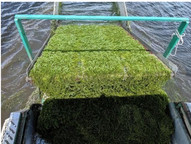
Figure 9. Thick, fresh-cut hydrilla being conveyed from the water column into the harvester.
