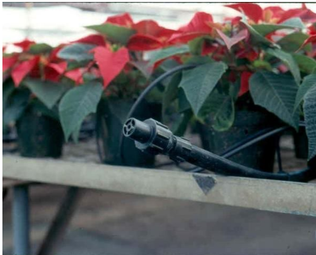
Figure 5. A low-pressure drain on the end of a pipe allows the pipe to drain rapidly when irrigation ceases.
