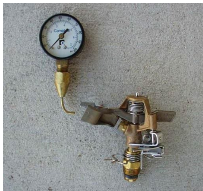
Figure 4. A pitot tube with pressure gauge is used to monitor pressure as water flows from the orifice.
