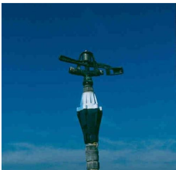
Figure 2. Appropriate nozzle operating pressure is achieved with a pressure regulator mounted below the sprinkler.
