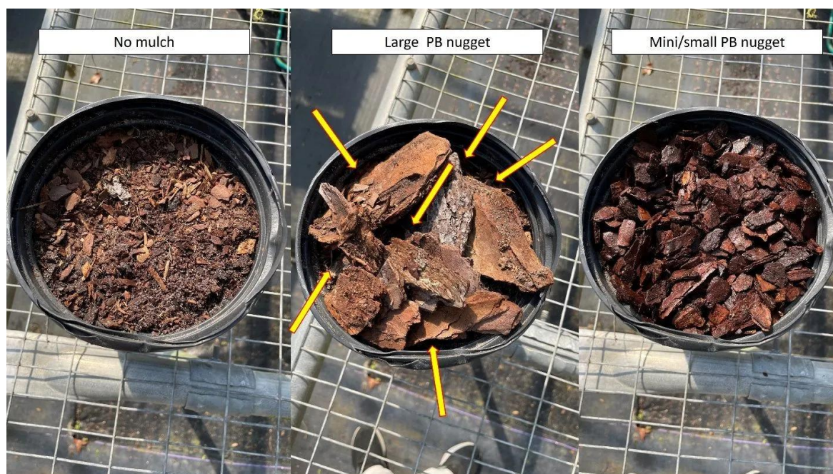
Figure 4. Comparison of no mulch (left), large pine bark nugget mulch (center), and mini/small pine bark nugget mulch (right). Yellow arrows in center photo indicate the gaps between the large pine bark nuggets.
