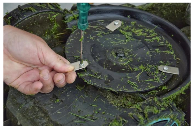
Figure 1. A close-up of three small, two-edged blades fixed to a spinning disk underneath an autonomous mower.
