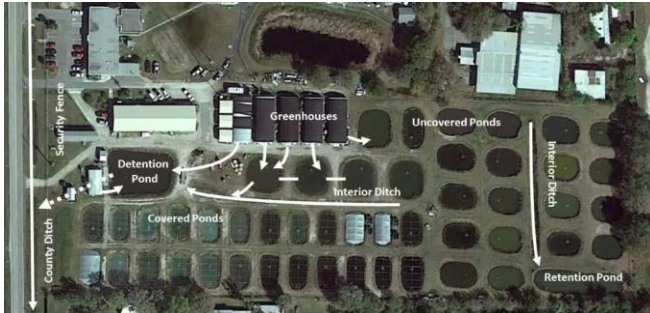
Figure 1. Representative fish farm layout. Water flow direction is indicated by arrows. Effluent from buildings and greenhouses flows into an interior ditch that empties into a detention pond. The detention pond discharges to the county ditch, the only surface water connection between the farm and the outside environment. Ponds are periodically dewatered by pumping into one of the interior ditches. The facility has security fencing, locked gates, and security lighting. Credit: Reprinted from Hill et al. (2016)
