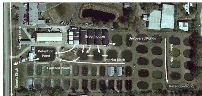
Figure 1. Representative fish farm layout showing several structural barriers used to prevent the release of organisms. Visible structural strategies include covers on ponds, a detention and retention pond, and a security fence surrounding the property. Further, riser-board control structures are found on both interior ditches before they flow to the detention or retention pond. Screening is also present on all vats and aquaria in the greenhouses. Water-flow direction is indicated by arrows. Credit: Reprinted from Hill et al. (2016)
