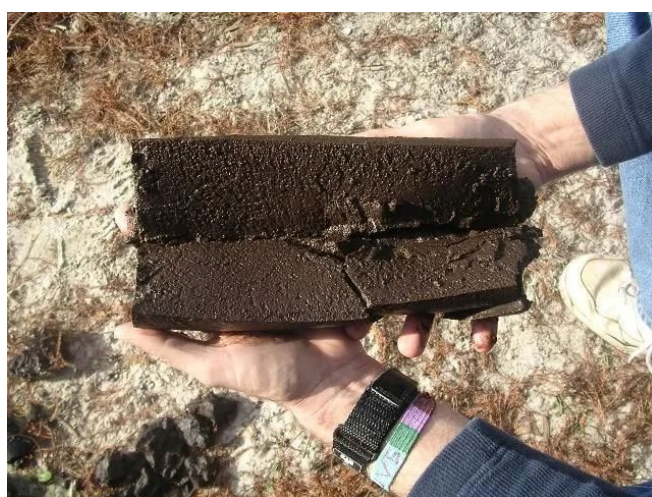
Figure 3. Mark Brenner holds a short section of a lake sediment core that was sliced lengthwise to reveal the consistency of deeper, consolidated, organic-rich mud deposits. The core was collected from Lake Lochloosa, north-central Florida.
