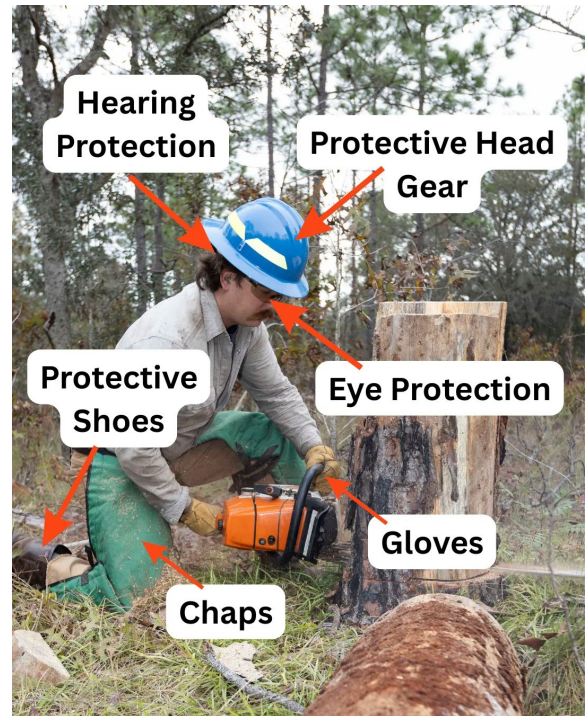
Figure 3. Personal protective equipment (PPE) is an important component of safe tree removal. Credit: Adobe Stock, Labels: Alyssa Vinson
