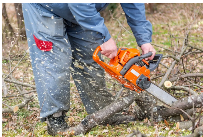
Figure 5. Chain saw use should be left to the professionals. If homeowners decide to use a chain saw, they should only work on the ground and with proper protective equipment—a hard hat with face shield, leg protection chaps, gloves, and hearing protection. This individual is lacking gloves and leg protection chaps.
