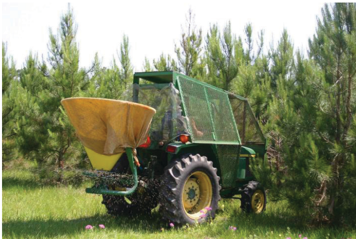
Figure 2. Mineral fertilizer application with a centrifugal fertilizer spreader. Note the cage on the tractor and the cover on the spreader, especially useful in younger stands.
