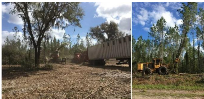
Figure 5. A whole tree chipping operation (left). A feller-buncher harvesting machine (right).
