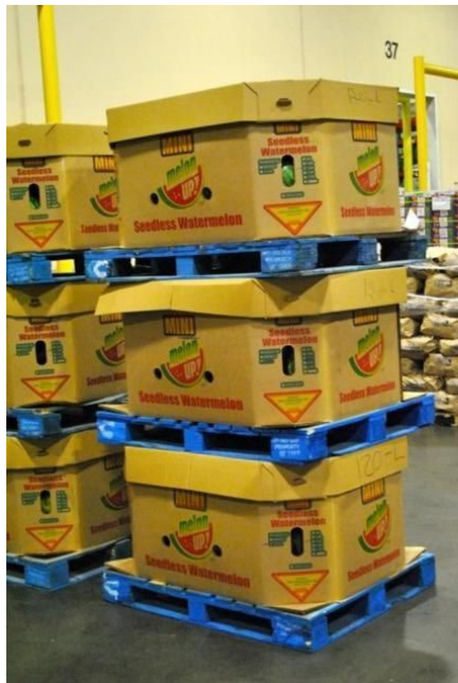
Figure 3. Corrugated fiberboard bulk bins are sometimes used to ship less perishable crops like potatoes or, as shown here, watermelons.
