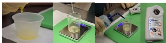
Figure 36. A pocket Brix-acidity meter. Note: Juice samples need to be diluted 1:50 to measure total acids. (Pocket Brix-Acidity Meter | ATAGO CO., LTD.) Credit: Sandra Matlack, USDA/ARS
