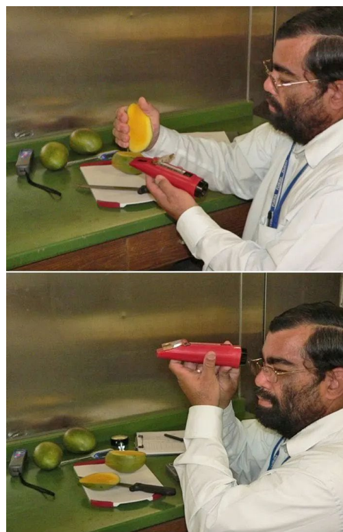
Figure 34. Measuring mango fruit SSC with a refractometer.
