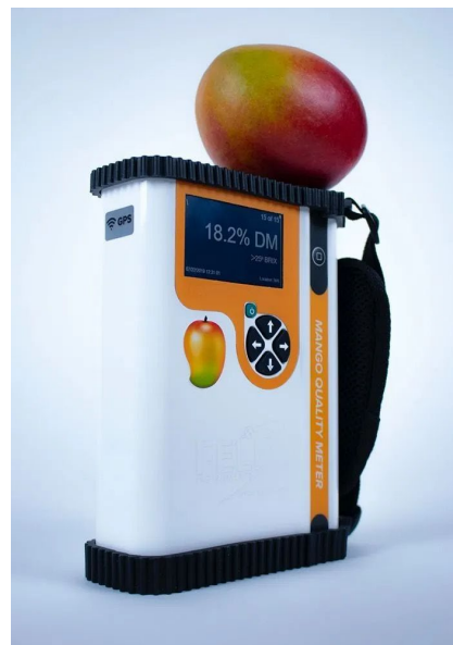
Figure 43. Handheld near infrared (NIR) instrument for measuring mango dry matter (DM) and soluble solids content (SSC).
