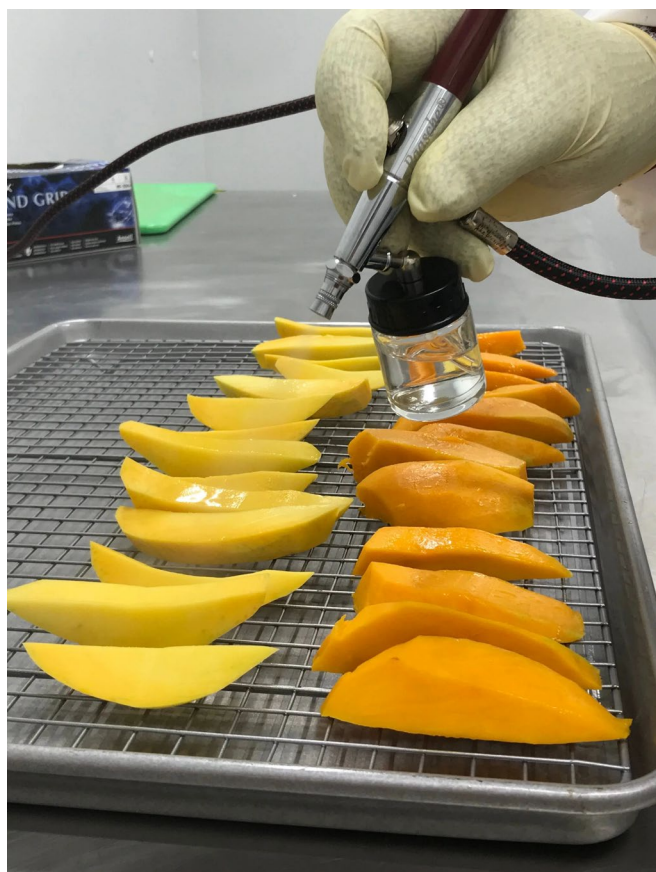
Figure 17. An airbrush being used in a lab experiment to spray fresh-cut mango slices with an anti-browning solution.
