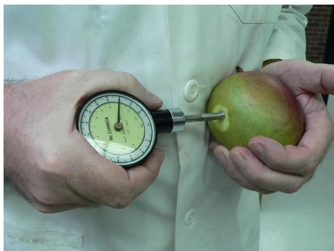
Figure 42. Measuring firmness with a handheld penetrometer.
