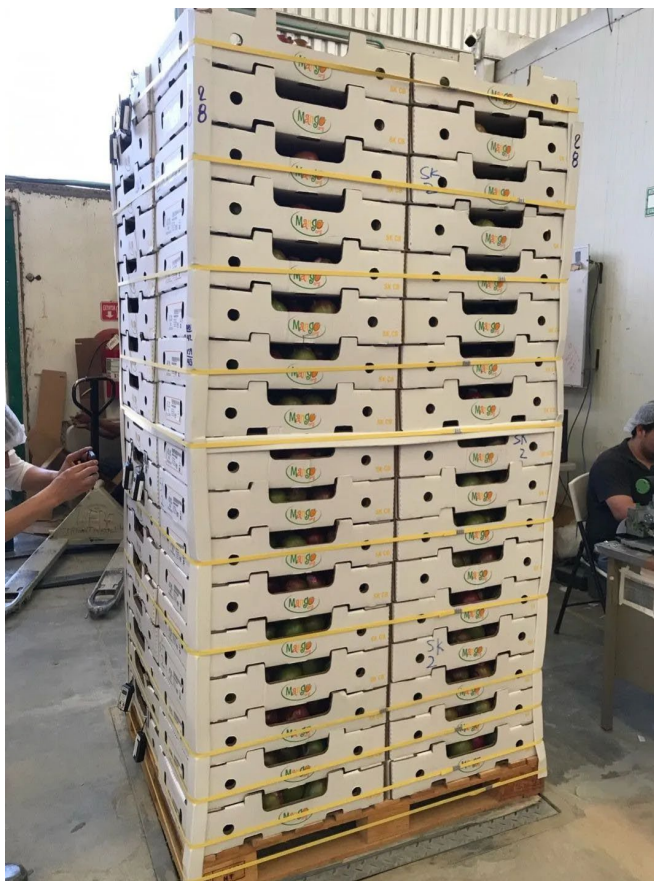
Figure 6. A pallet of properly designed 5-down mango cartons recommended by the National Mango Board ( https://www.mango.org/professionals/industry/mango-packaging-palletization/ ).
