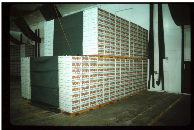
Figure 6-16. Forced-air cooling of palletized product. Credit: Mark A. Ritenour, UF/IFAS
