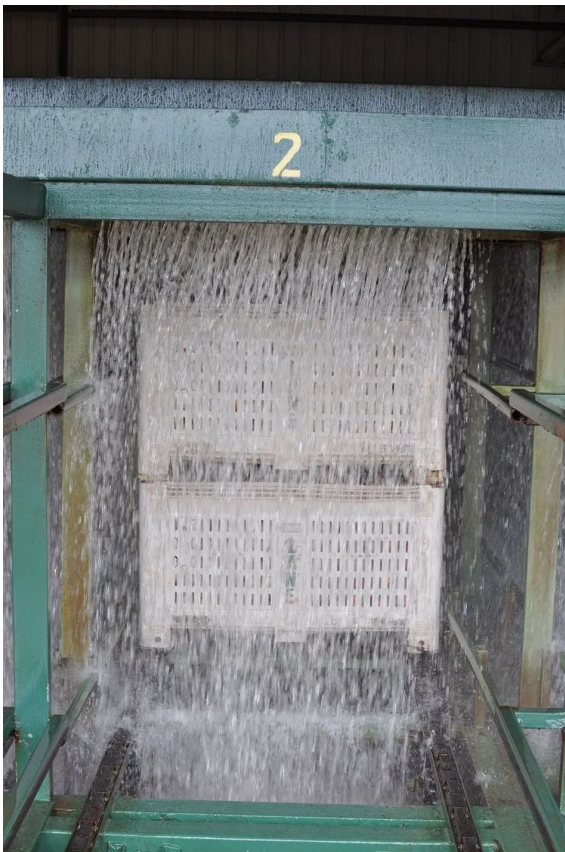
Figure 8-9. A continuous or tunnel hydrocooler in which the conveyor speed determines the duration of cooling. Credit: Jeffrey K. Brecht, UF/IFAS
