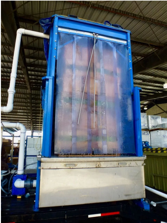
Figure 8-8. A stationary (batch) hydrocooler, which runs for a predetermined time to achieve 7/8 cooling. Credit: Jeffrey K. Brecht, UF/IFAS
