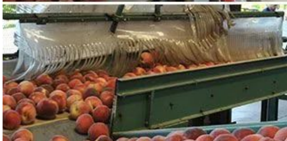
Figure 6-8. Counter directional soft bristle brushes (above) and plastic curtains (below) are used to decelerate peaches to reduce mechanical damage on the packingline.
