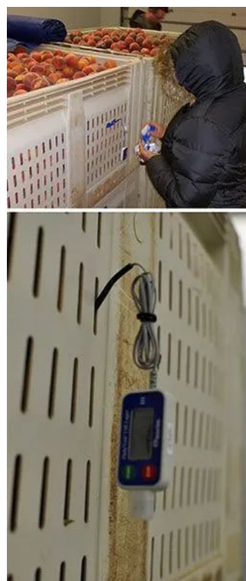
Figure 8-3. Probing fruit during cooling assures that the final temperature is reached. Here, a datalogger with its temperature probe is placed into a peach fruit during forced-air cooling.
