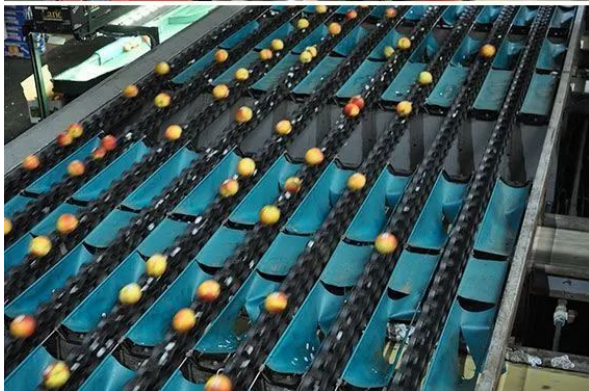
Figure 6-12. Fruit sizing being accomplished by a camera system (above) and a weight sizer (below). Credit: Jeffrey K. Brecht, UF/IFAS
