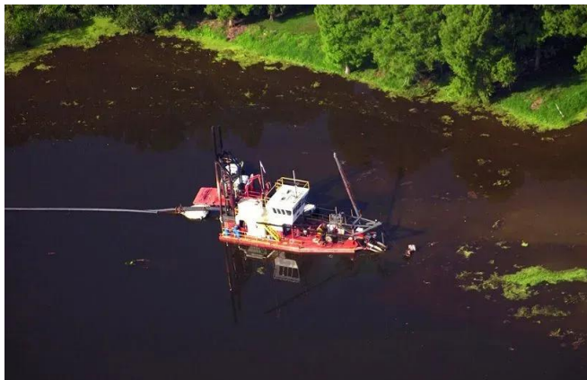
Figure 23. Dredging and pumping bottom sediments. Credit: Photograph by UF/IFAS Center for Aquatic and Invasive Plants.
