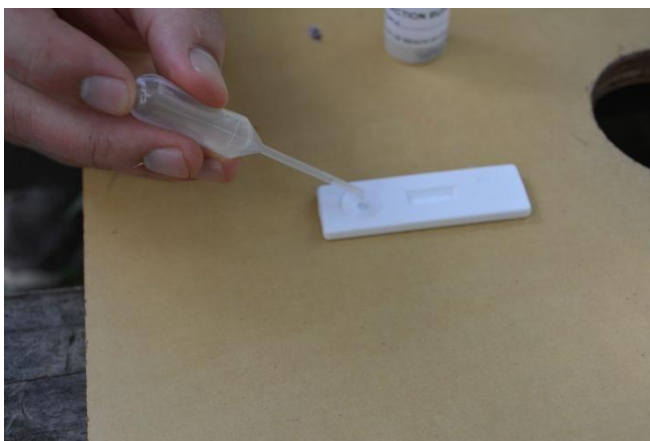
Figure 10. Squeezing two drops of the sample into the sample well with the pipette. Credit: C. Mueller, UF/IFAS Honey Bee Lab
