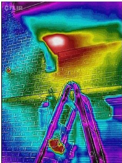
Figure 12. Locating a colony inside a structure using a thermal imaging camera.
