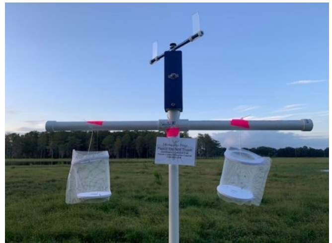
Figure 12. Caged mosquitoes and a rotating impinger with slides set up for a caged mosquito semi-field trial.
