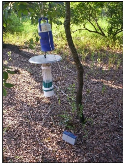
Figure 2. A CDC miniature light trap with container of dry ice hanging above it. These traps are used to attract and collect adult female mosquitoes seeking blood meal hosts.
