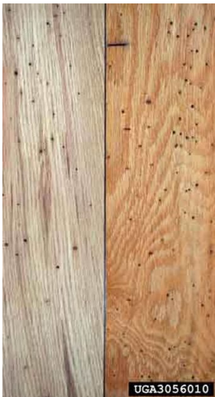
Figure 4. Damage (holes) caused by oak timberworm, Arrhenodes minutus (Drury), a primitive weevil.
