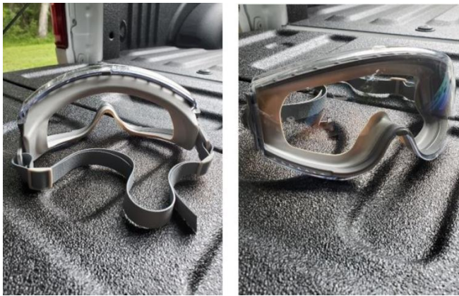
Figure 2. Neoprene safety goggles that seal around the face to better protect eyes from exposure to chemical splashing.
