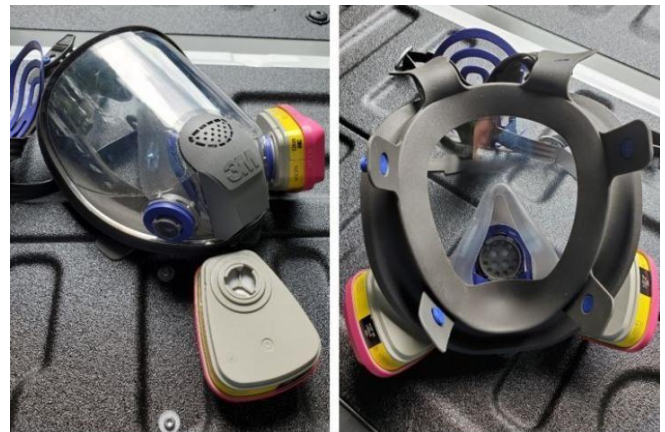
Figure 4. A full-face respirator, which qualifies as goggles, face shield, and respirator in one piece of equipment.
