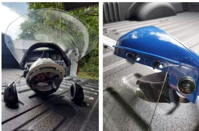
Figure 3. Hardhat face shield with ear protection incorporated and ratchet-style headgear highlighting quick-change levers.
