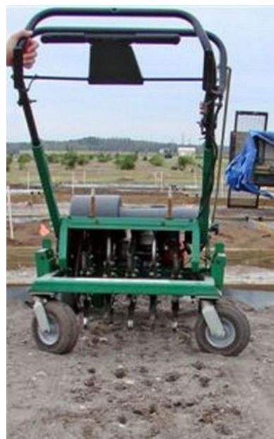
Figure 4. Plug aeration can be used to improve drainage in compacted soils with minimal effect on established plant roots or turfgrass.
