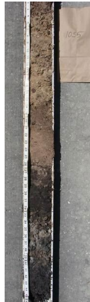
Figure 2. Removing a soil core or vertical slice from the disturbed soil to compare with the description of the native soil indicated on the site soil survey can provide information about the extent of soil disturbance during construction activities.
