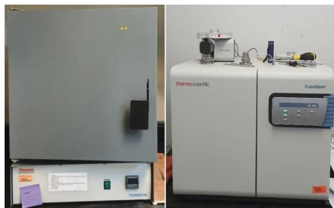
Figure 2. Incinerator for measuring C (left) and Dry Combustion Elemental C Analyzer (right).
