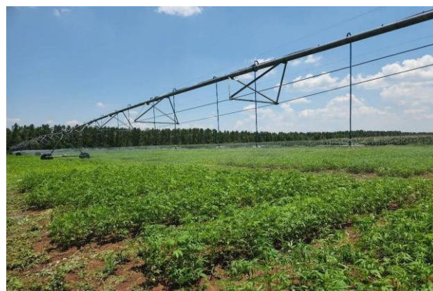
Figure 4. Pivot irrigation system with drop nozzles for hemp cultivation at the UF/IFAS Tropical Research and Education Center. Credit: Tanjila Jesmin, UF/IFAS
