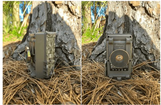
Figure 1. Camera trap with custom magnetic base that allows researchers to monitor wildlife movement through underground sewer systems.
